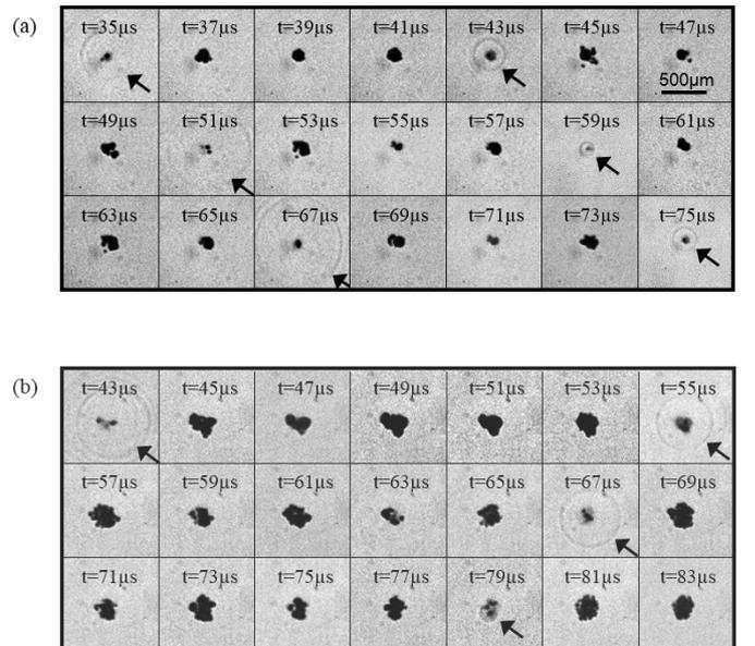
Fig. 2 Two image sequences illustrating cloud dynamics at HIFU  $\text{PA}_{\text{pp}} =$  (a)  $0.48$  and (b)  $0.62 \text{ MPa}$ . (a) represents five growth, oscillation and collapse (GOC) cycles, with shock-waves (arrowed) emitted periodically every  $\sim 8\mu\text{s}$ . (b) demonstrate three GOC cycles over an equivalent time, with shock-waves periodically every  $\sim 12\mu\text{s}$ .
