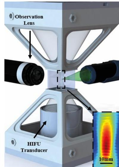
Fig. 1. The Sonoptic chamber was designed to house a 254 kHz HIFU transducer, the focus of which (at 64mm from the front face) is centrally located within a central glass section. Cavitation activity is nucleated via a 6-8 ns laser pulse (green). *Inset bottom right* is a normalized axial scan of the acoustic focus, generated in-situ by fibre optic hydrophone, confirming the HIFU field is not affected by the chamber housing.
