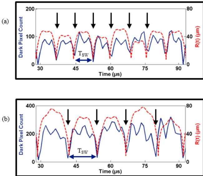
Fig. 3(a, b). Dark pixel counting algorithm (blue) used to analyze high speed camera data and quantify clouds dynamics at HIFU  $PA_{\text{pp}} = 0.48$  and  $0.62 \text{ MPa}$ . Rayleigh-Plesset model results for a single bubble (red dash), under equivalent acoustic driving and of selected quiescent radius,  $R_0$ .
